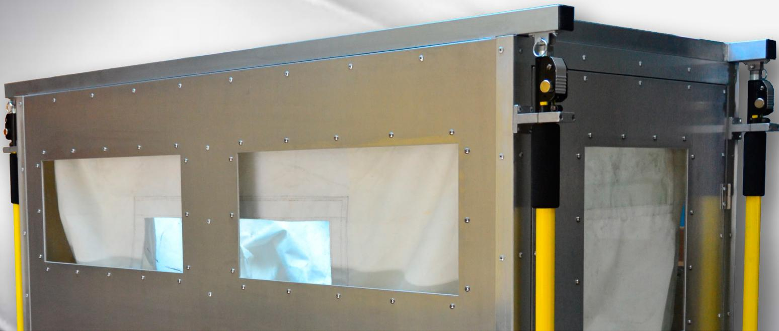
The Kontrol Kube HardPanel Containment system is an ultra durable solution for mobile containment. Built from aircraft grade aluminum, the Kontrol Kube HardPanel is designed for daily repeated use. The HardPanel is a highly configurable design that can accommodate a HEPA filtered DOP compliant negative air machine on the inside or on the outside of the unit. This enables the user to expand or contract the footprint of the unit depending on the space that is available.
